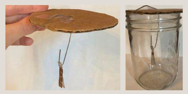
Experimental setup showing how the cardboard, paperclip, and aluminum foil strips should be arranged and placed on the jar.
